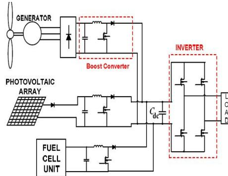
Figure 1: Hybrid system with multi-connected boost converter
