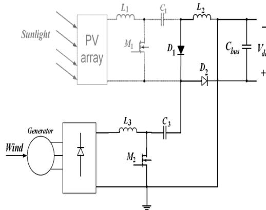
Figure 4: Only wind source is operational (SEPIC)
