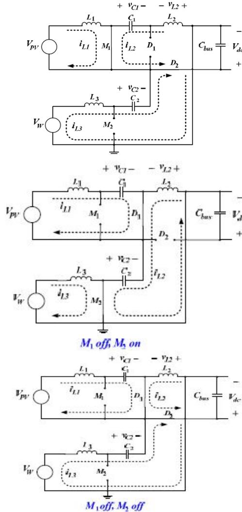
Figure 6 (I-IV): switching states within a switching cycle
