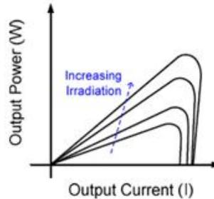
Figure 9: PV cell power characteristics
